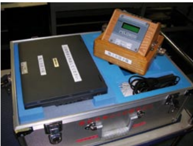
Vaisala BAROCAP® Digital Barometer PTB220TS in a portable oak case.
