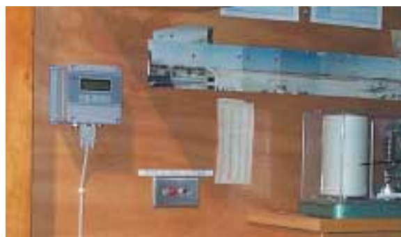
One of Vaisala's PTB220 digital barometers installed at London, Ontario, Canada. Vaisala supplies electronic station barometers to replace the mercury barometers currently used for weather observations throughout Canada.
