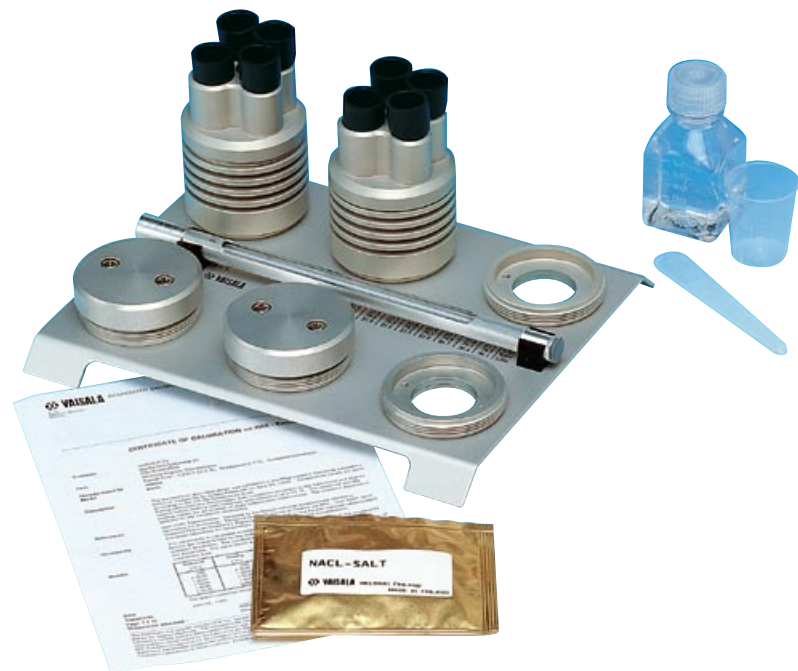
Vaisala Humidity Calibrator HMK15 - an example of a saturated salt bath device.
