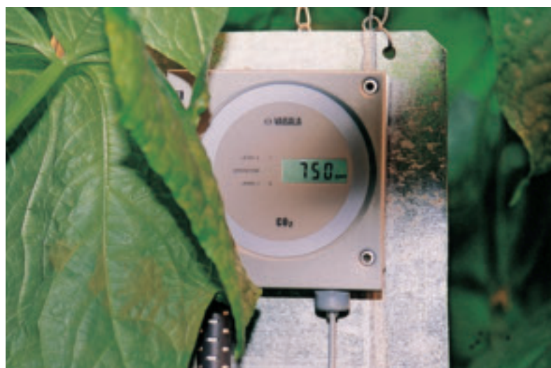
The Vaisala GMT222 gives continuous and accurate measurements of CO 2 concentrations - basic information for the operation of the fertilization system.
